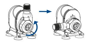
Remove impellor from the pump motor. Wash parts with fresh water carefully.
