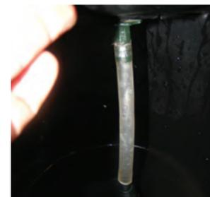
Then using the silicon hose push fit it to the hosetail and attach the other end to the pump to work out the distance needed. Different size pots will need different lengths of hose so it's important to get it right. Once you know the correct length, detach the pipe from the pump side and cut the hose with a pair of scissors carefully.
