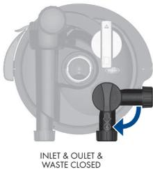
**5** Replace and rotate dosing chamber cap.
