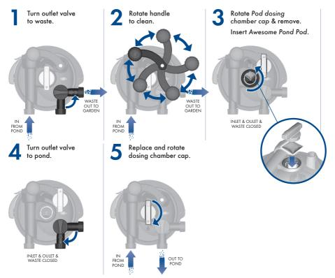
**NOTE:** A maximum of 10 Awesome Pond Pods can be fitted into the dosing chamber at any one time, this is sufficient for a pond with a volume of 1500 gals. If a higher amount is needed, the dose should be split in half and dosed over subsequent days to allow the pods time to dissolve.
