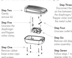
Step Three Disconnect the air line between the diaphragm/ flapper valve and
